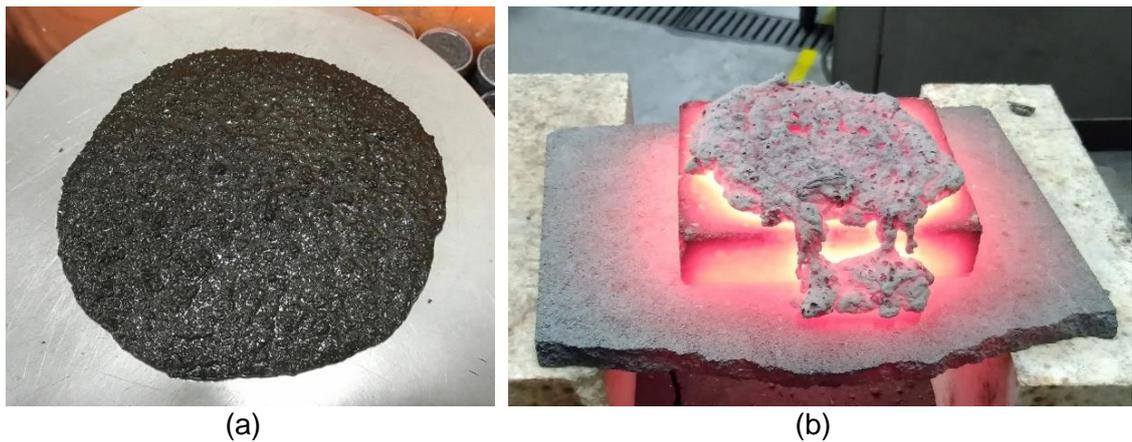
Figure 1 – (a) Self-flow test for self-flow repair mix; (b) Thermal flow at 1,000°C.
