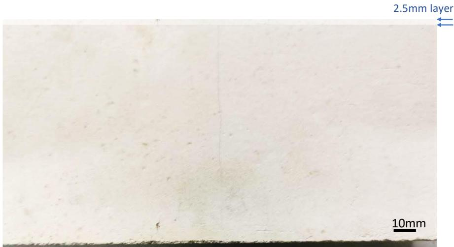
Figure 10: Photo of cross-section of insulating foam with 2.5mm Al<sub>2</sub>O<sub>3</sub> layer deposited by laser. Note the cracking perpendicular to the Al<sub>2</sub>O<sub>3</sub> layer.
