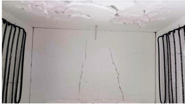
Figure 2: Typical cracking on hot face insulating lining of furnaces.
