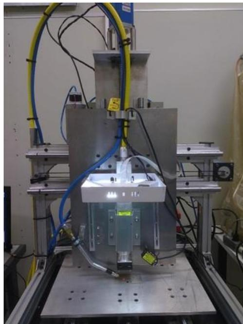
Figure 5: System with intelligent control, based on algorithms of computational vision, able to evaluate the surfaces to be worked for customized applications.
