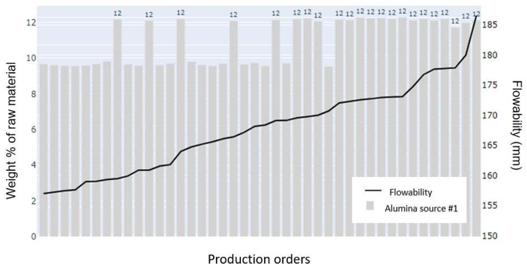
Figure 4 – Weight % of alumina source #2 plotted against flowability for different production orders, arranged in order with increasing flowability. Formulations with higher weight % of the raw material usually present higher flowability.
