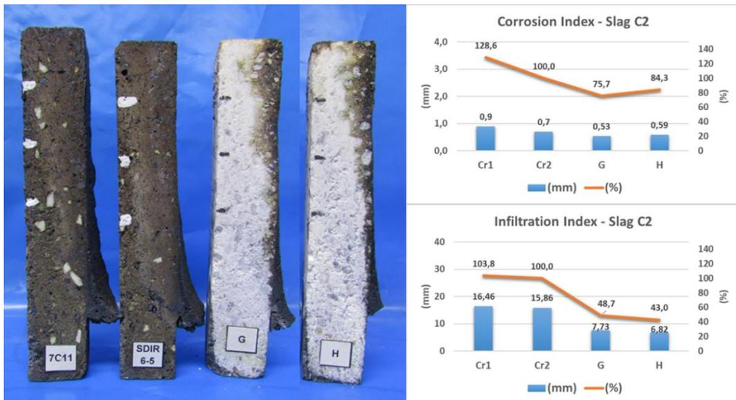
Figure 5 – Results for chromium containing commercial bricks and formulations G and H submitted to a corrosion by CaO/Al<sub>2</sub>O<sub>3</sub> slag C2.
