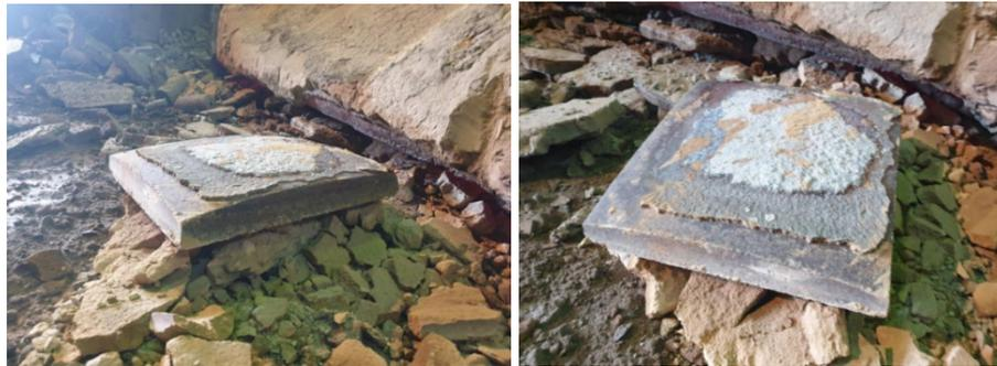
Figure 13. Condition of Spheric impact pad after casting of 32 heats (5760 tons of steel)
