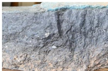
Figure 15. Break (realised in laboratory) of Spheric impact pad in area of direct impact of stream of casted steel after casting of 32 heats (5760 tons of steel)
