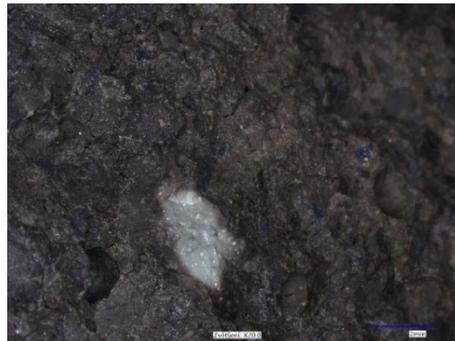
Figure 16. Material structure of the impact pad after use (magnification x20)
