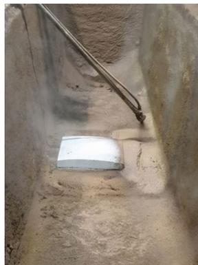
Figure 14. Installation of Spheric impact pad in tundish
