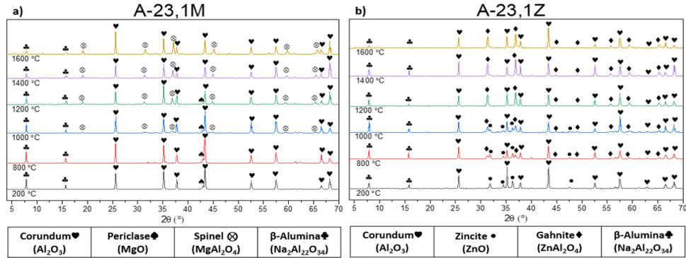
Figure 1: Qualitative X-ray diffraction evolution for  $\text{Al}_2\text{O}_3\text{-MgO}$  (a) and  $\text{Al}_2\text{O}_3\text{-ZnO}$  (b) systems.
