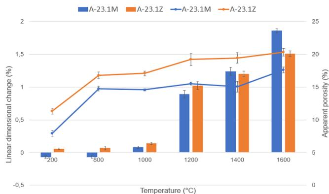
Figure 2: Apparent porosity and linear dimensional change after different firing temperatures.
